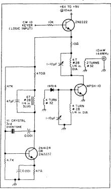
Figure 1. Schematic of the 10 mW transmitter.
